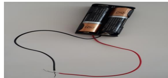
Photograph 2. A Short Circuit
